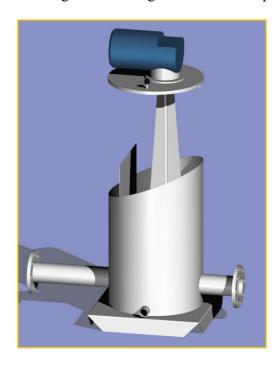
Siljan Allards supplies flocculation reactors, the capacities are selected to suit thickeners/dewaterers of different capacities; In the table below, the sizes and retention times of each flocculation reactor are shown.
